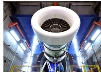
ESSAI DE FATIGUE RÉACTEUR
